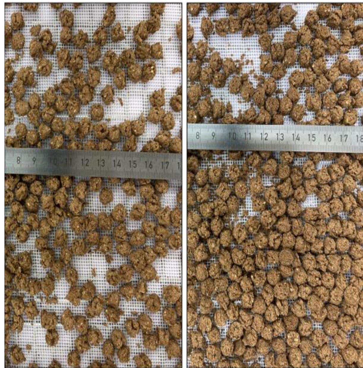
Figure 13: Comparison of product samples without (setting 20, left) and with oil (setting 21, right).
